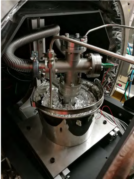
Figure 3: Static gas extraction prototype during thermal-vacuum testing
