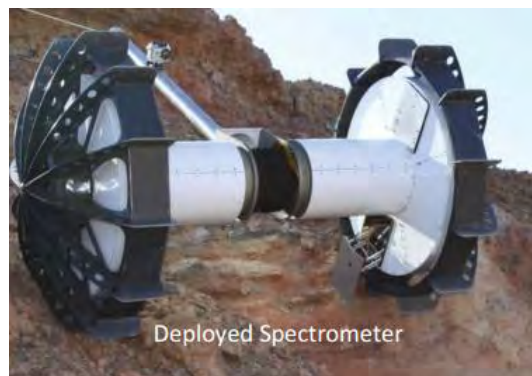
Figure 2. The Axel rover taking spectroscopic measurements on a slope of 40° (figure from [14]).
