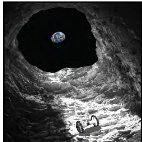
Figure 1. A representation of the Axel rover rappelling into a lunar pit as part of the Moon Diver mission. This mission's exploration of mare pits with potential subsurface void spaces would address numerous top-priority lunar science goals.
