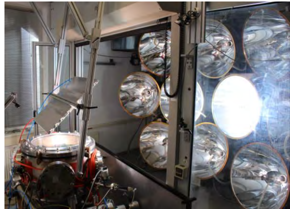
Fig. 1: Solar 3D printed setup for vacuum printing
