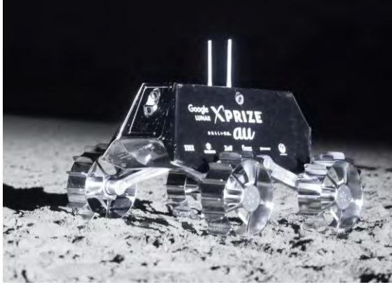
Figure 2: SORATO rover's camera imaging test in the field.
