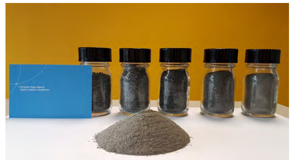
Fig. 2 – Image of EAC-1 simulant material in various grain sizes, the development of which has been spearheaded by Spaceship EAC.
