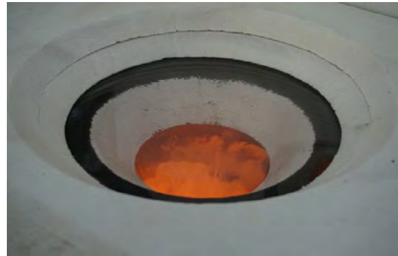
Fig. 2: Fluidized bed (“solar lava lake”) at 900°C.
