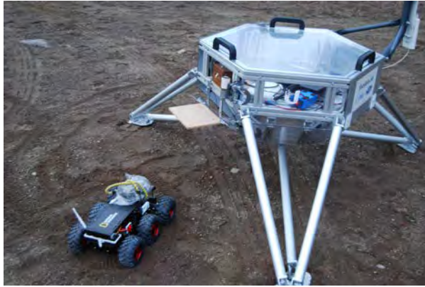
Fig. 4, ILEWG ExoGeoLab lander with remotely controlled USB4000 spectrometer and rover
