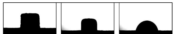
Figure 2: Drop shape analysis of JSC-2A using HSM technique.
