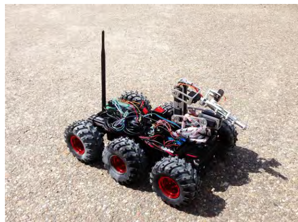
Figure 3: The Rover [6] made by Mateusz Krainiski is controlled via WiFi signal by ExoHab crew in order to explore extraterrestrial sights.
